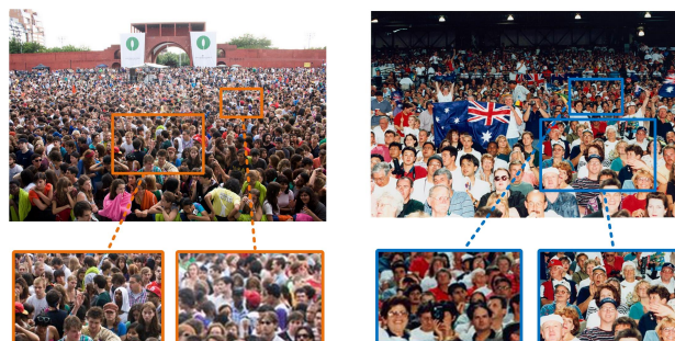
Fig. 1: In dense crowd images, regions of different scales exhibit high visual similarity if we resize them to certain sizes. This indicates the importance of scale invariance in crowd counting.
